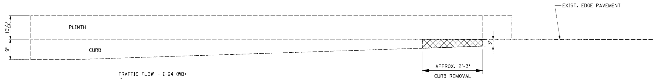
SAFETY CURB PLAN - REMOVAL LIMITS
